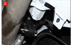
To remove the original exhaust the system requires cutting in two places.
